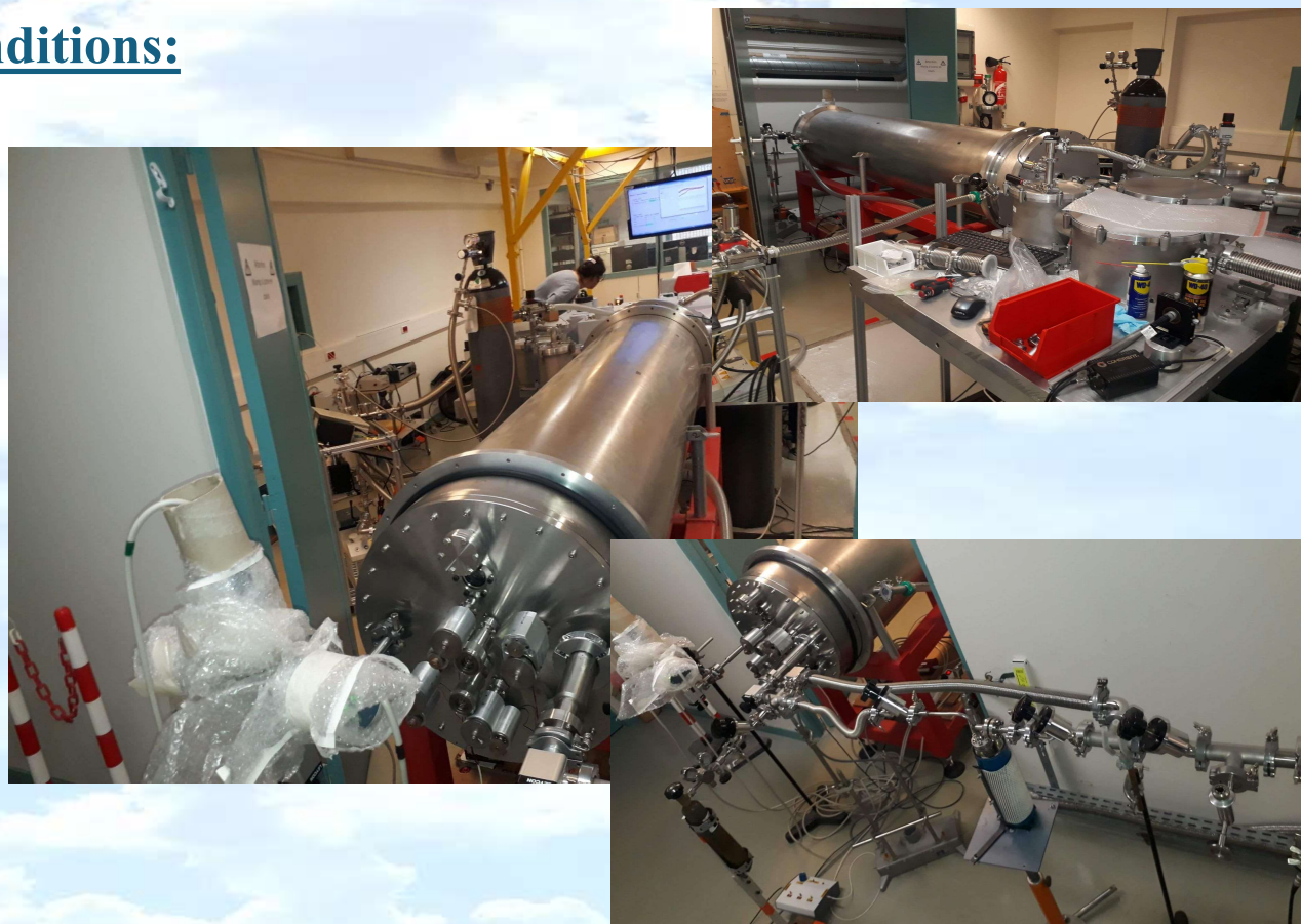
The 125HR TF spectrometer coupled with a 2 m multi-pass cell
